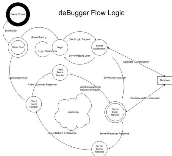
Figure 7 - deDebugger Flow Logic used to show the cycle of information being passed between *Client* and *Server*
